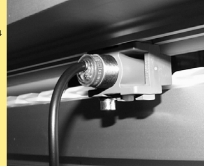
Bracket for horizontal proximity switch \varnothing 18 \text{ mm} XKPB 18 H Acetal resin. Including screw, T-slot nut and washer
